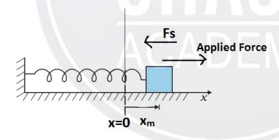
The work done by the spring force for an extension of xm is
